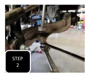
**Step 2** Un-bolt the sway bar end link at the lower control arm.
