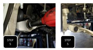
**Step 5** Remove the bolt attaching the strut to the lower control arm and allow the lower control arm to hang by the ball joint.
