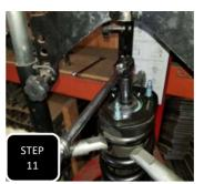
**Step 10** Install the provided lower coil seat and then transfer over the factory bump stop.
