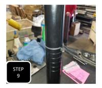
**Step 9** Install the retaining clip onto the desired groove using retaining ring pliars and make sure it fully engages into the groove.
