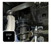
**Step 6** Un-bolt the strut at the top by removing all 3 nuts and remove the strut.
