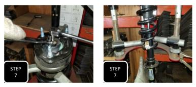
**Step 7** Compress the coil using a strut compressor and remove the nut at the center of the strut top. **NOTE: IF THE THREADS HAVE ANY RUST, SPRAY WITH WD-40 AND LET SOAK FOR A FEW MINUTES.**
