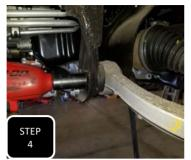
**Step 4** Un-bolt and remove both alignment cam bolts attaching the lower control arm to the frame.
