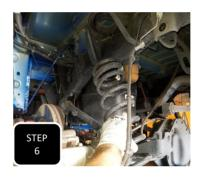
**Step 5** Make sure the floor jack has pressure under the diff. Now, unbolt both shocks at both ends and remove.
