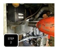
**Step 2** Unbolt the trac bar from the axle and separate
