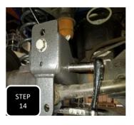
**Step 14** Insert the provided 3/8" bolt through the drilled hole and tighten.
