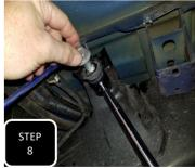
**Step 8** Jack up the axle until the coils make contact with the upper coil seat. Make sure that the coils both seat properly, then install both of the provided shocks with the
