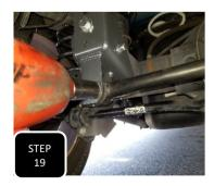
**Step 19** Re-install the wheels and lower the truck to the ground. Jump on the bumper a few times to settle the suspension and then tighten up the trac bar while the truck
