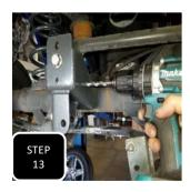
**Step 13** Either mark the side hole and remove the bracket or using the side hole of the provided trac bar bracket as a guide, drill a 3/8" hole through the factory bracket.
