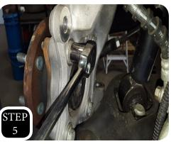
STEP 4: Remove the rotor, then unbolt and remove the abs sensor from the back side of the spindle, then support the sensor up and out of the way so it does not get damaged.
