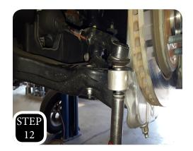
**STEP 12:** Attach the tie rod to the spindle and tighten.
