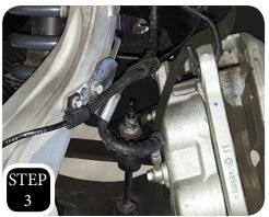
STEP 3: Unbolt the brake line bracket and the ABS bracket from the spindle. Next, unbolt the brake caliper and support it so it is out of the way. (NOTE: NEVER ALLOW THE CALIPER TO HANG BY THE BRAKE LINE).
