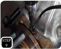
**STEP 8:** Re-install the factory wheel bearing using the factory hardware
