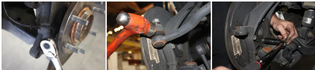
7. Discard dust shield, it will not be used with the new lift spindle.
