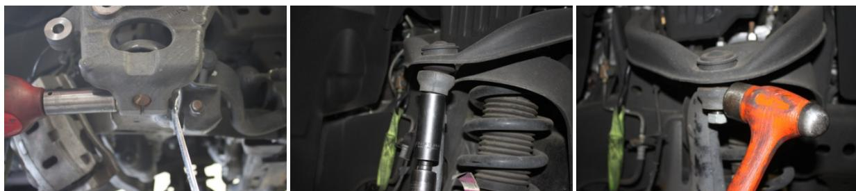
11. Slide Maxtrac spindle over lower ball joint and install factory bolt and nut (don't tighten yet)
