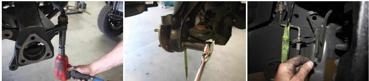
17. Install ABS sensor back into unit bearing and then tighten.
