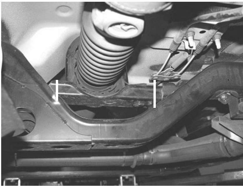
4. Locate the #615399 Carrier Drop Down Bracket, and the supplied hardware. The drop bracket has a taper (slant) built into it, which requires the side designated with the **R** to face the rear axle. Attach the drop bracket to the carrier bearing with the hardware and torque to 40lbs. Lower the drive shaft into the crossmember now.
