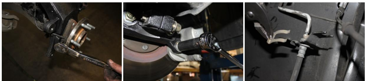
20. Unbolt factory brake line at frame and caliper. Then install new steel braided brake line and tighten. Install provided clip at the frame bracket next to the shock tower.
