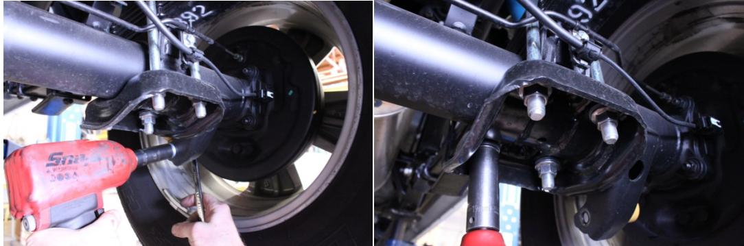
6. Install the lift block on the factory spring pad with the angled part towards the front of the vehicle.
