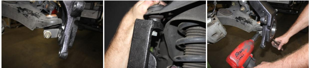
13. Install tie rod from the top down on Maxtrac spindle and then tighten
