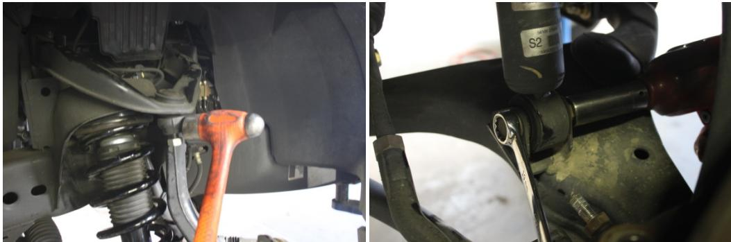
4. Remove the strut from the vehicle and mount it in a bench vise, and install the Maxtrac strut spacer kit. Torque fasteners to OEM specification. Note the shape of the spacer, the strut will be rotated 180 degrees when installed.
