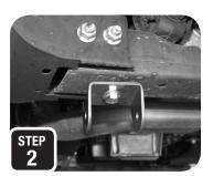
**STEP 2:** Loosely attach each of the two angled u-strap plates to the back of the rear cross member using the provided  $\frac{1}{2}$ -13 x 1  $\frac{1}{2}$ " bolts. *Note: ensure that the angled u-strap plates are angled outward.*
