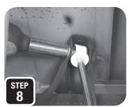
$\triangle$  IF THE SHOCKS ARE MOUNTED UP-SIDE-DOWN, THEY WILL NOT WORK PROPERLY AND CAN GO BAD  $\triangle$
