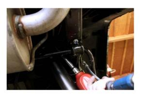
17. Remove bolt that holds track bar to axle housing, remove both coil springs.
