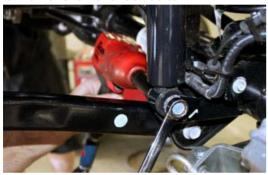
5. Remove Coil Springs and isolator.
