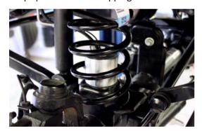
11. Install Maxtrac Shock using original hardware at axle, and new hardware at the shock mount.
