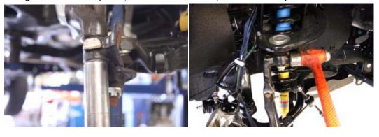
11. Guide ABS line down between the new spindle and lower ball joint/ steering stop plate. Slide lower ball joint into the double sheer mount & attach upper ball joint to new spindle, tightening nut on ball joint, align cotter pin hole & install OEM cotter pin.
