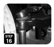
**<u>NOTE:</u>** Once both sides have been installed, all air will need to be bleed from the system and the vehicles toe will need to be adjusted before driving to an alignment shop.
