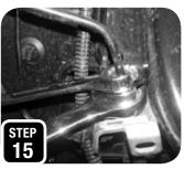
**NOTE:** 2015 MODELS WILL USE THE BRAKE LINE WITH THE THREADED ADAPTOR. 2009-2014 MODELS WILL NOT USE THE THREADED ADAPTOR.
