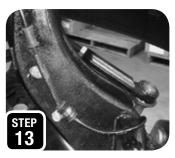
**STEP 14:** Unbolt the brake line bracket at the frame to provide enough slack to allow you to bolt up the brake caliper. Then re-install the rotor & the caliper, and tighten.
