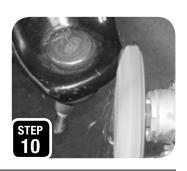
STEP 10: On 2009-2014 models, the whole front of the arm will need to be ground down about ¼" NOTE: IF YOU DON'T WANT TO GRIND, YOU CAN ALSO REMOVE THE
