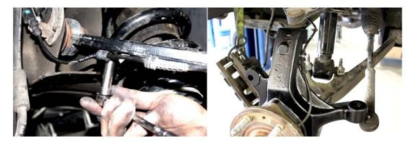
13. Install the extended brake lines using the provided clips, install the frame side first and allow fluid to run through the line before installing the caliper side. This will ease the bleeding process.
