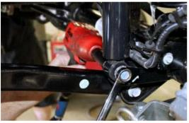
5. Remove Coil Springs and isolator.
