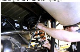
18. Set welded nut plate in thru top of the frame in coil bucket. Install rear spacer w/ the new 1/2" bolt and lock washer. Install spring isolator.
