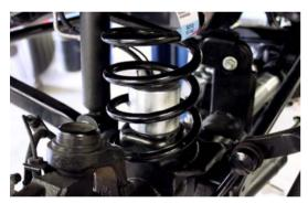
11. Install Maxtrac Shock Extenders using original hardware at axle, and new hardware at the shock mount.
