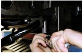
6. Grind lip on front bump stop holder, approximately 1/3 of the front diameter.
