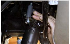
22. Install extended brakeline bracket using original bolt at the frame. Use the new bolt washers, and nuts at the lower hole.
