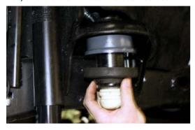
9. Install Coil Springs, with bump stop spacer loose. After spring is in place, tighten bump stop spacer with self tapping bolt.
