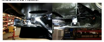
**6)** ONCE THE METAL SKID PLATE IS TIGHT, RE-INSTALL THE FRONT PLASTIC SKID PLATE. IT WILL NEED TO BE STRETCHED SLIGHTLY TO RE-ALIGN WITH THE MOUNTING HOLES.
