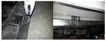
5) REINSTALL THE SKID PLATE USING ONE ½" SPACER AND A PROVIDED BOLT AND WASHER AT EACH OF THE FRONT MOUNTING HOLES. AND THE LONGER PROVIDED BOLTS WITH TWO ½" SPACERS AND A WASHER AT EACH OF THE TWO REAR SKID PLATE MOUNTING HOLES.
