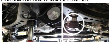
**4)** BEND THE TWO FRONT GUIDE TABS ON THE METAL SKID PLATE SO THAT THEY CAN NO LONGER ENGAUGE IN THE HOLE ON THE FRAME.
