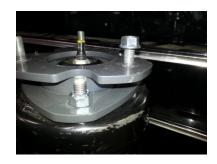
\*WITH THIS SPACER INSTALLED, THE SPINDLE WILL COME INTO CONTACT WITH THE COIL WHEN THE SUSPENSION IS AT FULL DROOP. THIS WILL "NOT" OCCUR UNDER NORMAL DRIVING CONDITIONS, ONLY WHEN THE VEHICLE IS LIFTED COMPLETELY OFF THE GROUND
