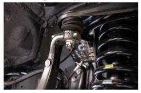
11. Reattach sway bar end links, and put wheels back on the vehicle.
