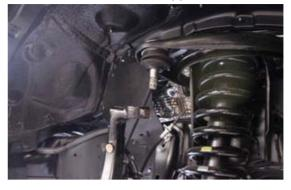
6. Pry down lower arm to remove strut
