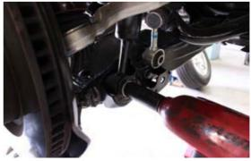
9. Reattach upper strut mount with provided nuts and tighten
