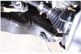
Remove ABS guide on back side of upper arm so as not to be torn when arm is pried down.
