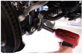
3. Remove upper strut mounting hardware
