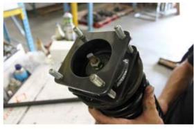
8. Reattach lower strut mounting hardware
