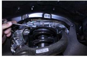
4. Remove lower strut mounting hardware
