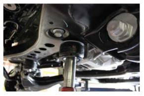
SKID PLAT SPACER INSTALLED
