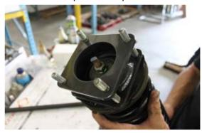
8. Reattach lower strut mounting hardware
