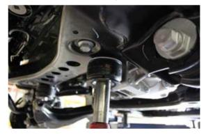
SKID PLAT SPACER INSTALLED
