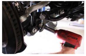
3. Remove upper strut mounting hardware
