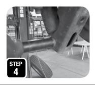
STEP 4: Loosen the u-bolts at one side, then remove the u-bolts on the other side. NOTE: "LOOSENING THE OPPOSING U-BOLTS ALLOWS FOR EASIER ALIGNMENT OF THE BLOCK BEING INSTALLED"
