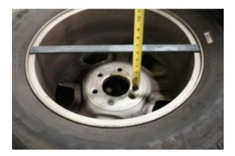
In the example below, you can see the wheel mounted, and the possible clearance issue that arises. This is the area that you have to worry about touching other parts of the suspension such as the steering knuckle, tie rod ends, etc. In this case, there's plenty of room on our test vehicle.
