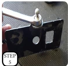
**STEP 5:** The rear sensor plate will need to be installed as soon as the axle is flipped and the U-bolts are ready to be installed. Remove the mounting ball from the original plate and re-attach it to the new plate using the provided 6mm nut.
