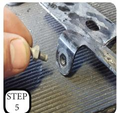
NOTE: If installing a 4" or 6" drop, the ball will be installed in the furthest hole.
