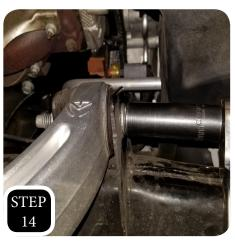
**STEP 14:** Once both arms are installed, and the truck is back on the ground, tighten down both control arms.
