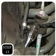
**STEP 13:** Re-ttach and tighten the tie rod then attach the ABS guide clip.
