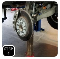
**STEP 5:** Jack up the truck and support under the frame rails with jack stands. Keep an adjustable jack under the control arm for height adjustment.
