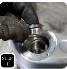
**STEP 1:** Install the tapered shank and the shank topper into the control arm bearing.
