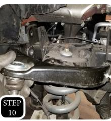
**STEP 10:** Unbolt both control arm mounting bolts and remove the arm.
