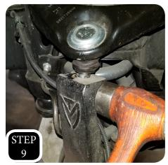
**STEP 9:** Loosen the upper ball joint nut, but do not remove. Break the nut loose by hitting the side of the spindle with a hammer. The nut will catch the spindle, then remove the nut and separate the upper control arm from the spindle.
