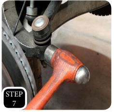
**STEP 7:** Loosen the tie rod nut, then break loose with a hammer and separate.
