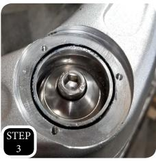
**STEP 3:** Apply a little bit of grease to the supplied "O" ring and place it in the machined groove on the control arm.
