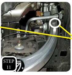
**STEP 11:** Attach the new control arm to the frame using the factory hardware. Only loosely tighten the hardware, do not fully tighten until the truck is on the ground and the suspension has settled.
