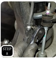
**STEP 8:** Unbolt the ABS guide clamp and move the line out of the way so that you can access the upper ball joint nut.
