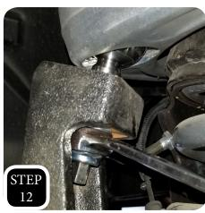
**STEP 12:** Attach the control arm to the spindle using the provided M14 nut and washer, then tighten.
