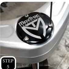
**STEP 4:** Align the "MT" aluminum dust cap and attach using the supplied M4 button Allen bolts.
