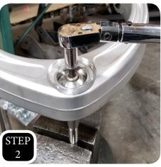
**STEP 2:** Thread in the M10 Allen head bolt and torque to 30 ft/lbs.
